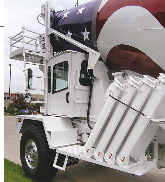
It's up, in and down to the low-slung driver's seat inside the cab, which is constructed of stainless steel to resist cleaning chemicals. The mixer barrel's forward end tapers its way over the cab, funnel and chute.
