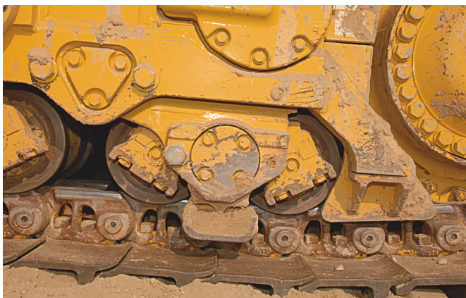
The D155AX-6 has an overall more robust undercarriage than its predecessor, with a wider gauge and more track-on-ground. The Dash-6 undercarriage also uses Komatsu's "K-type" bogies, which incorporate a pair of bottom rollers housed in an oscillating frame that is suspended only at one end.
