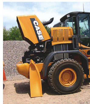
One-piece flip-up hood, a lift-up panel over the tire, and a removable inner tire fender give the E Series "best-in-class" maintainability, says Case.
