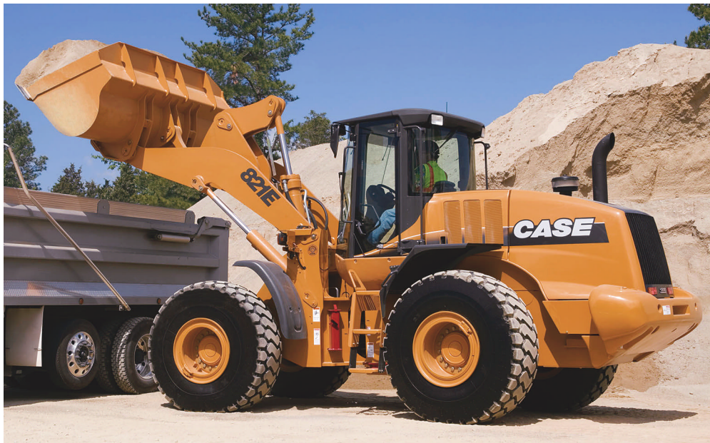
Case 821E allows operators to match power to fuel economy. In high-production activities such as aggregates operations, they may choose maximum power at all times for high breakout force and fast cycling.
