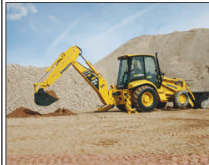
The Utility Division of Komatsu America has refined models in its backhoe-loader line with addition of available joystick controllers for
