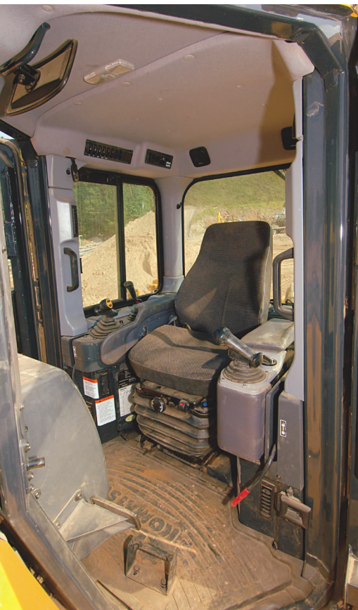
Both the Dash-6 and the Dash-5B feature Komatsu's single-lever, Palm Command Control System for steering and blade control. The Dash-6 also uses a new variable-displacement, axial-piston pump in its implementation hydraulic system, which operates at a considerably higher pressure than the gear pump in the Dash-5B.
